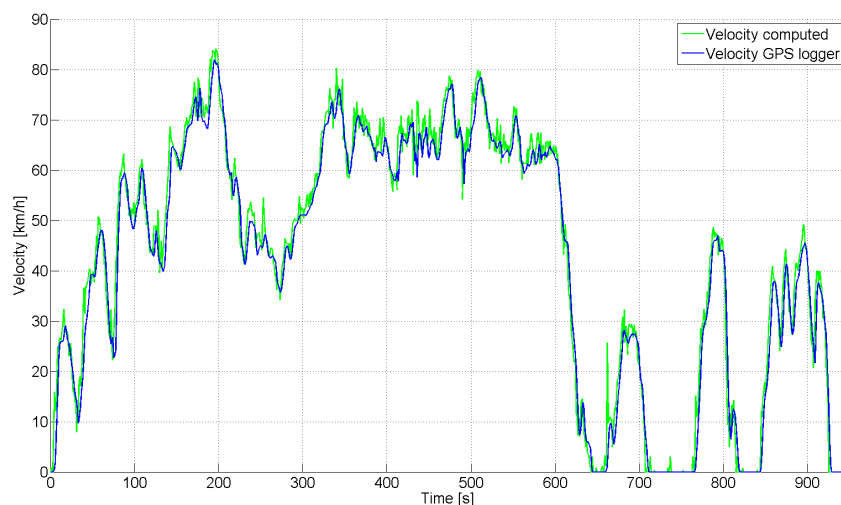
FIGURE 5.4: Comparison of speed values from GPS logger (blue) and speed computed on basis of sample point's GPS coordinates (green)
