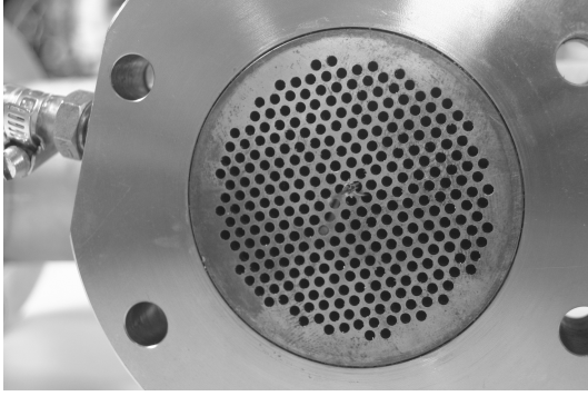
Figure 3: Cold heat exchanger with a room temperature water income on the left.
