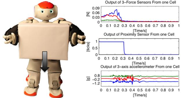
Fig. 1. Exploring objects properties by NAO. While object is within its arms it detects the stiffness of the object via output of the force sensors and during sliding, it distinguishes different surface texture and classifies objects having various weights via accelerometer feedback.
