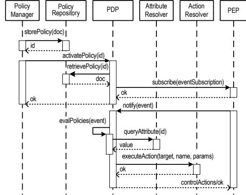
Figure 1. Policy enforcement sequence diagram
