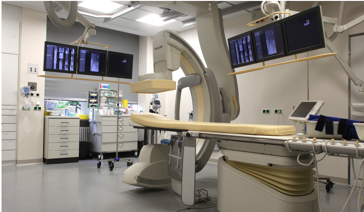
Figure 6.1.: The core component of a C-arm system is the C-shaped mount carrying an X-ray tube (bottom) and a digital flat-panel detector (top). Due to its shape, the assembly can be rotated around an iso-centre. (Courtesy of José Gardiazabal.)
