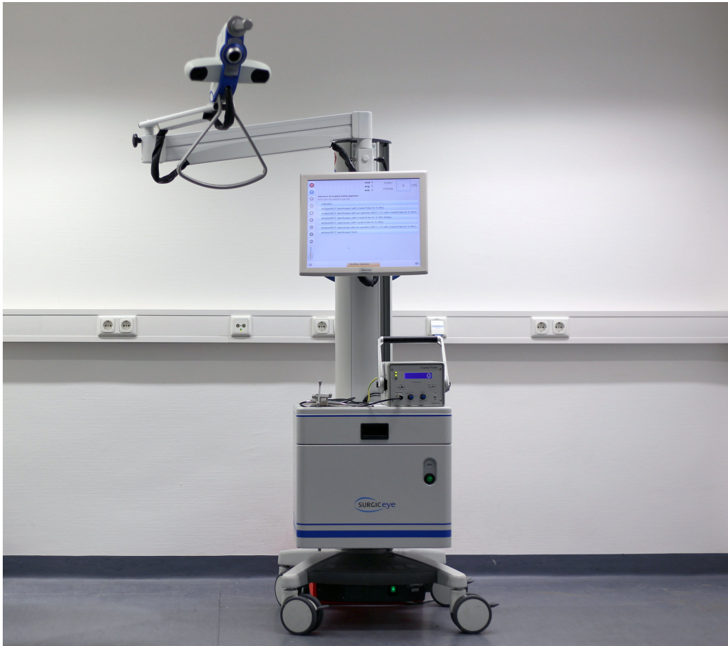
Figure 7.1.: The freehand SPECT system uses an optical tracking system (top left) to track position and orientation of a \gamma -radiation sensor (centre, on cart, with cross-shaped tracking target) which is hand-guided by a surgeon. Like this, measured counts are related to sensor perspectives, thus enabling tomographic reconstruction. (Courtesy of José Gardiazabal.)
