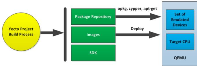
Fig. 4. Build process of Yocto Project [11]
