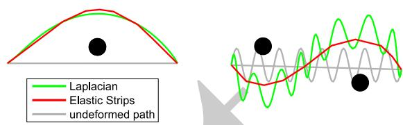
**Fig. 10** Comparison between Elastic Strips and LTE in the presence of obstacles (black)
