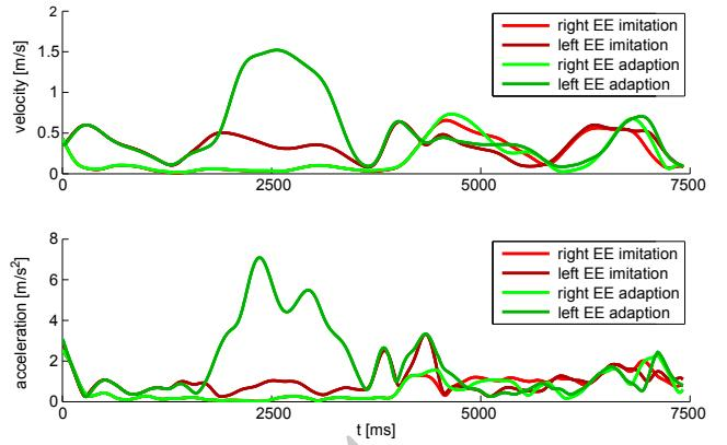
**Fig. 12** Motion imitation task: Endeffector velocity (top) and acceleration (bottom) over time for the robotic movement reproduction and adaption
