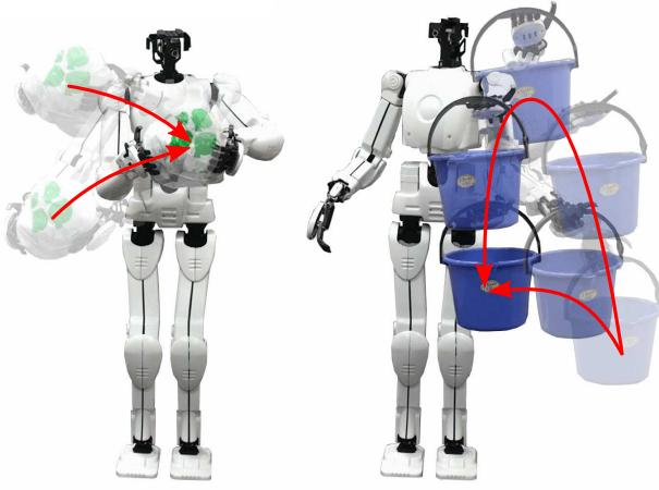
**Fig. 1** Application of Laplacian trajectory Editing to deform a given reference motion while maintaining its local shape: Adaption of a bimanual task from different start positions maintaining a fixed spatial distance between both hands (left) and modification of a one-handed pick-and-place task to avoid a possible obstacle (right)
