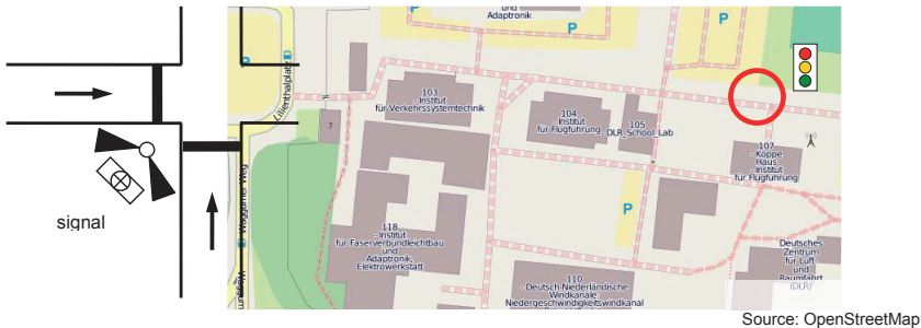
Figure 4: The test site is a simple intersection consisting of two crossing one-way streets, each signaled by a separate signal group (left). The intersection is located at the non-public property of the DLR in Braunschweig (right).
