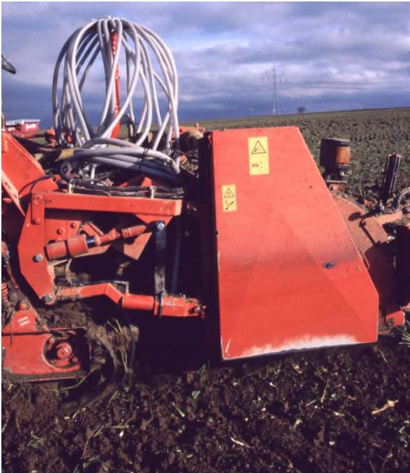
Broadcast seed in front of lifting unit with pneumatic seed distributor
