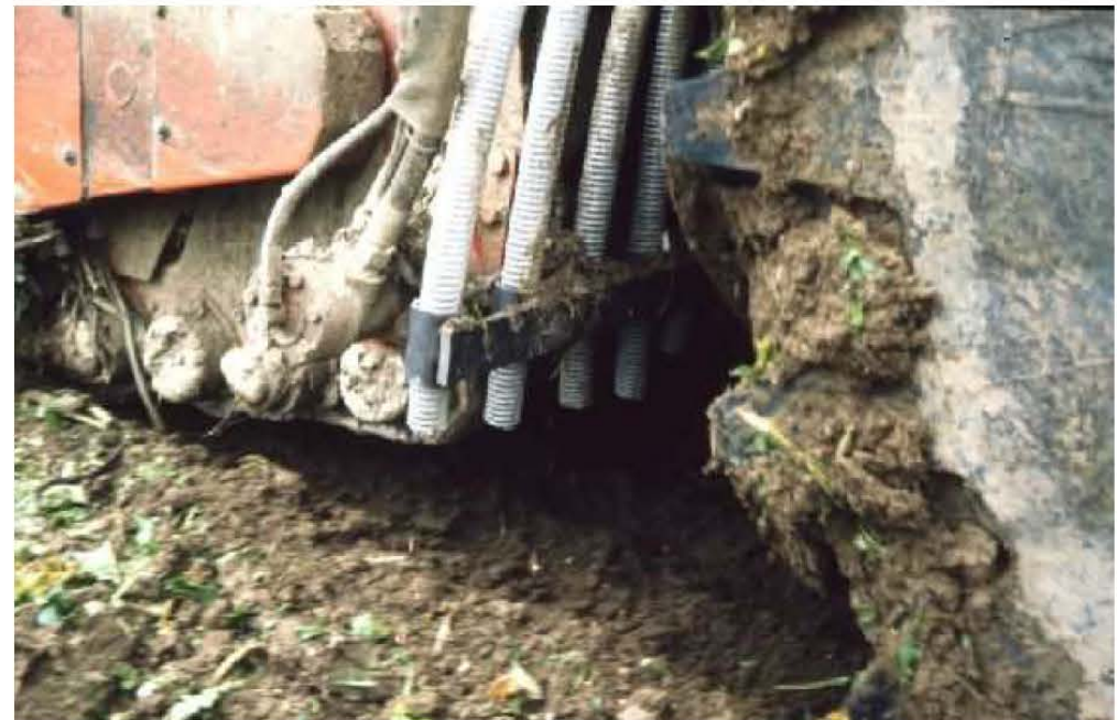
Broadcast seed in back of lifting unit with pneumatic seed distributor
