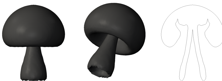
Figure 9.21: Position of merged bubbles (left and middle) and interface in the x_1x_2 -centerplane (right) at time t = 0.2 s of the coalescence.
