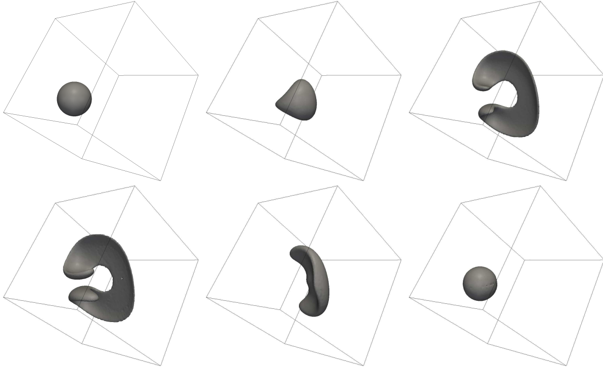
Figure 8.7: Three-dimensional deformation of a sphere at times t = 0, 0.25, 1, 1.5, 2.5 and 3 .
