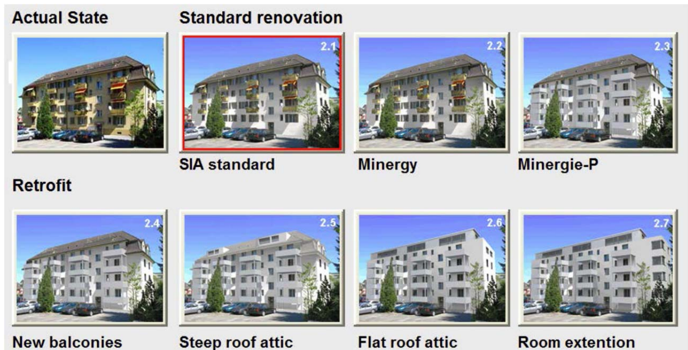
Figure 2-4 Illustration of different quality levels of retrofit, starting with the existing building top left up to a total refurbishment including extensions. Image is taken from the Retrofit Advisor (Zimmermann [12])
