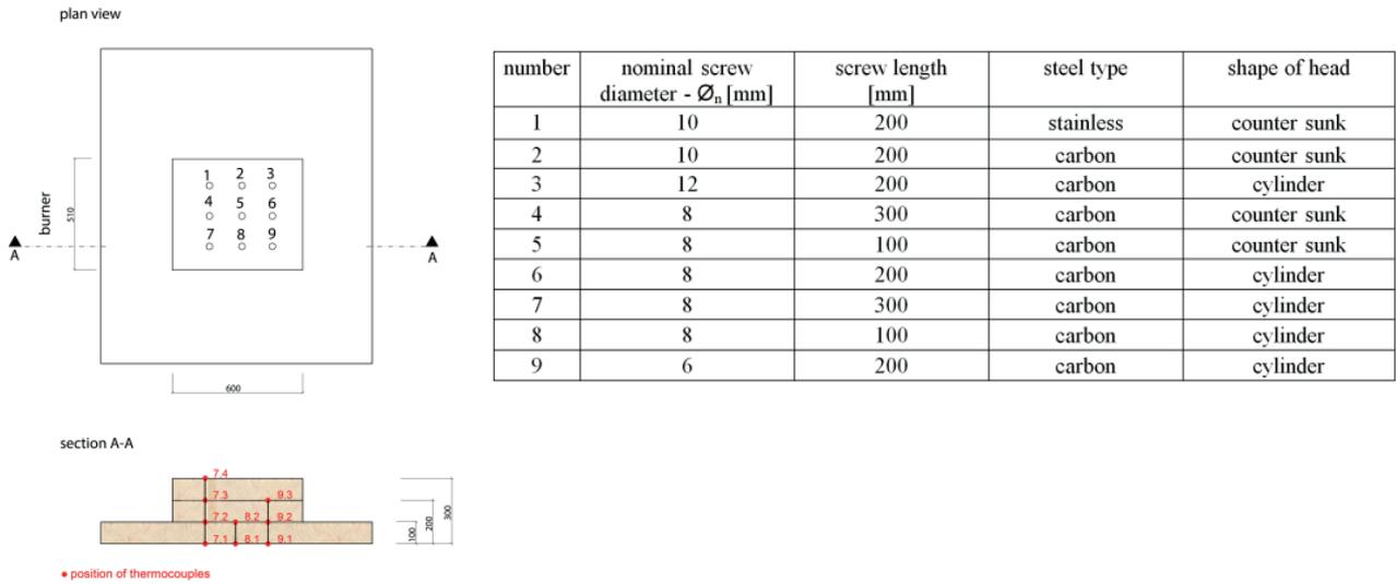
Figure 4. Position of full thread screws in the CLT ceiling element with corresponding measurement points.
