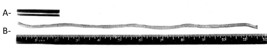
Figure 2.4.: Image of \alpha -U deformation. After around 3000 cycles at temperatures between 50 and 550°C, the solid bulk (A-) of highly textured uranium has grown around six times in size (B-) [15].
