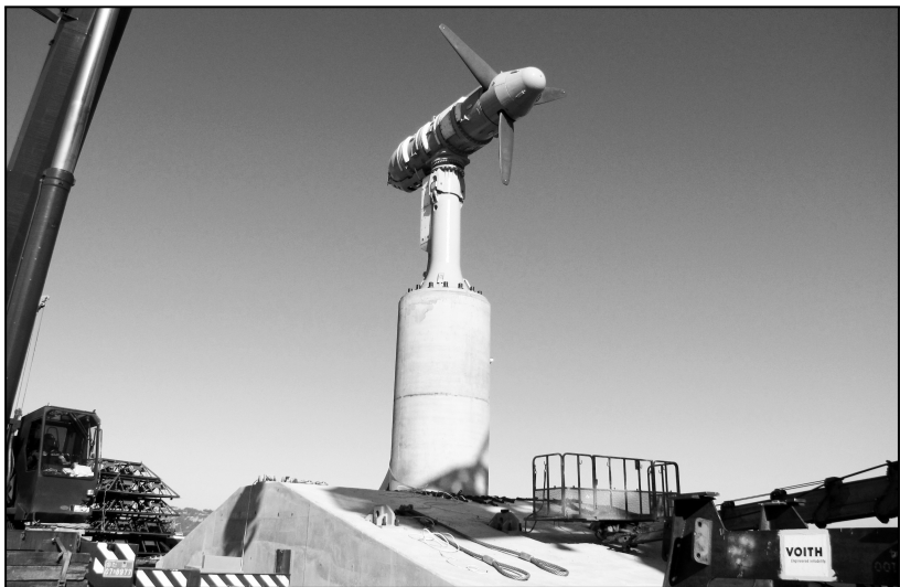
Figure 3.7: Prototype support structure and 110kW tidal turbine [RENETEC, Voith Hydro].
