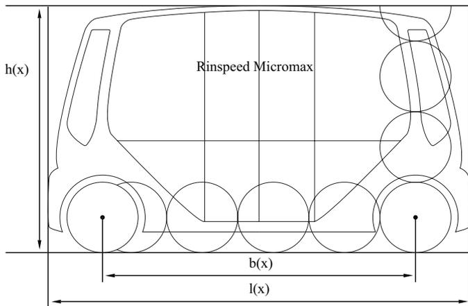
Fig. 10. Exterior proportion analysis of the vehicle concept Rinspeed Micromax.
