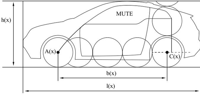
Fig. 8. Exterior proportion analysis of the vehicle concept MUTE.
