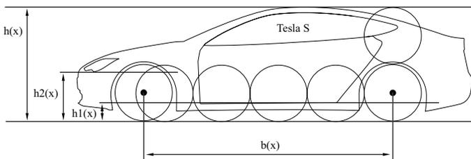
Fig. 6. Exterior proportion analysis of the Testla S.
