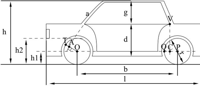
Fig. 1. Key features used for the analysis of exterior vehicle proportions [1].
