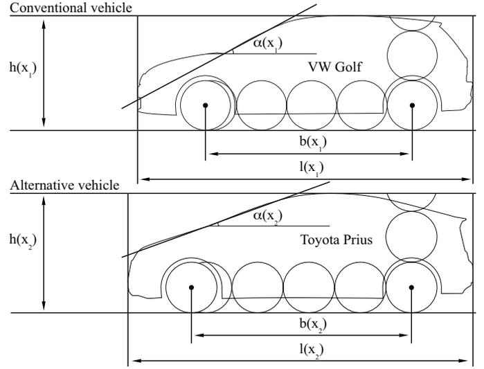
Fig. 2. Comparison between a conventional ( $x_1$ ) and hybrid ( $x_2$ ) vehicle.
