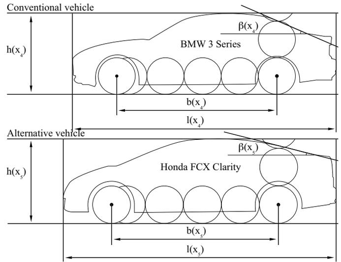
Fig. 7. Comparison between a conventional ( $x_4$ ) and fuel cell ( $x_5$ ) vehicle.
