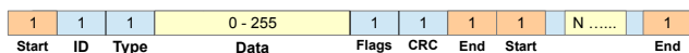
Fig. 6. The data structure of the High Speed Communication frame. Each sub-frame is separated with a start and stop unique word using 8/10b encoding.
