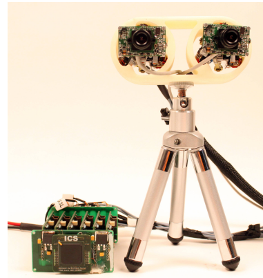
Fig. 9. High speed vision tracking system. This setup is used to demonstrate the FPGA can control 6 piezo motor in parallel. On the left is the electronics, where the FPGA is interfaced to 6 OEM piezo motor control boards and interfacing of 6 incremental encoders.
