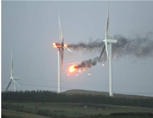
Figure 1.1: Exploded wind turbine in Ardrossan, North Ayrshire, Scotland due to high winds and problems with the emergency shutdown British Broadcasting Corporation [21]
