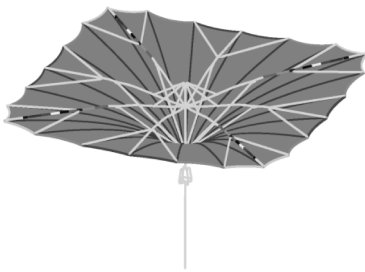
(a) A lightweight umbrella structure from a collaboration with SL Rasch, http://www.sl-rasch.de
