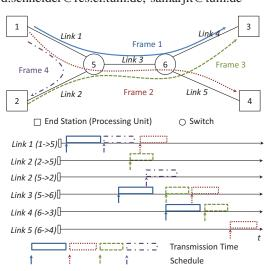
Fig. 1. An example of time-triggered traffic in switched Ethernet network.
