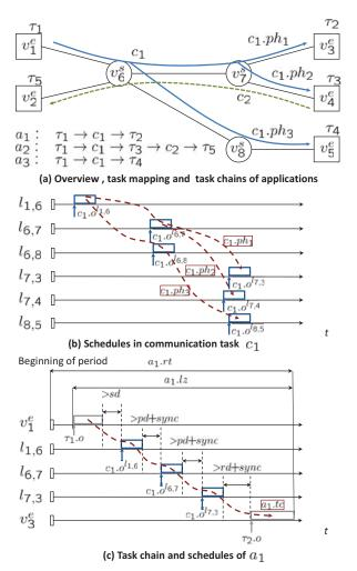
Fig. 2. Example of a distributed system of applications  $a_1$  to  $a_3$ , application tasks  $\tau_1$  to  $\tau_5$  and communication tasks  $c_1$  and  $c_2$ .
