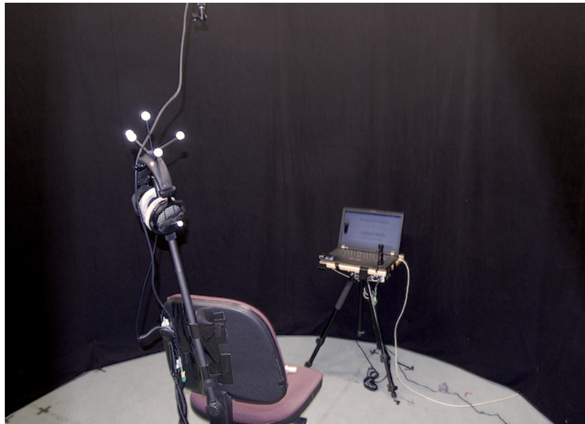
Figure 5.1.: Fleece mounted at the ceiling to serve as cylindric projection surface for the laserdot.
