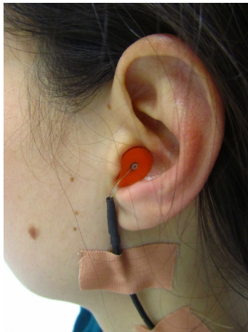
Figure 3.1.: Imprints and microphone placement for the HRTF measurements.
