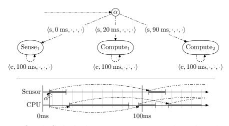
Figure 3.7.: Strictly Cyclical Jobs in Power Management Plan and Timeline View
