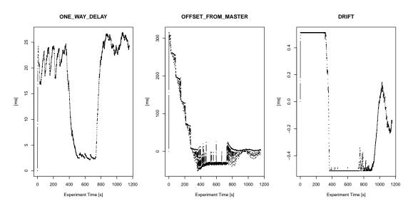
Figure 6.10.: Test Case 1; regular PTPd control system values for Subsystem 1. Subsystem is idle except for cyclically flushing these values to the Linux PC.
