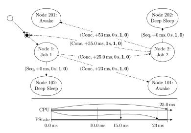
Figure 5.4.: Functional Chain Set for Validation of Deep Power States
