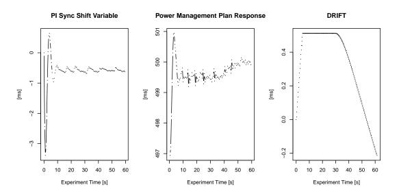
Figure 6.13.: Test Case 3; transient response of the plan control system for Subsystem 1. In the beginning, the plan scheduler response is aligned with the plan behavior, after second 40, the reponse starts to shift to 500 ms due to to the drift value for compensation of the offsets.
