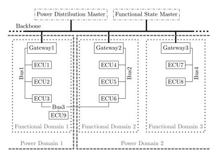
Figure 3.11.: Illustration of technical hierarchy from Barthels et al. (2012a). The vehicle is subdivided into different functional domains which are interconnected by a backbone. Different sets of subsystems form different power domains (high voltage, low voltage, ...).
