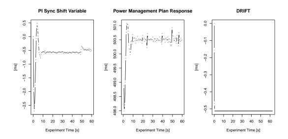
Figure 6.15.: Test Case 3; transient response of the plan control system for Subsystem 2. Sync shift, drift and response pretty much constant during the phase of systematic compensation of the offsets.
