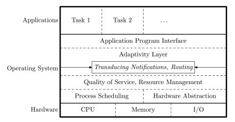
Figure 3.8.: Adaptivity is Modeled as Transducing Inputs to Plans
