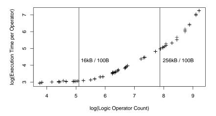
Figure 6.9.: Results from synthetic randomized sequential logic operator test as conducted as part of Gleixner (2013). Logarithmic execution time in  $\mu$ s over logarithmic signal and operator count. Vertical lines depict theoretical optimistic L1 data cache and L2 cache boundaries of the underlying platform.
