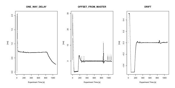
Figure 6.12.: Test Case 3; regular PTPd control system values for Subsystem 1. The initial offset from master is small. Slight disturbances may be observed at around 300 and 800 s Experiment Time.
