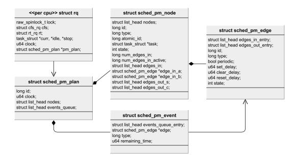
Figure 5.3.: Power Management Plan Data Structure as Held Within the Scheduler
