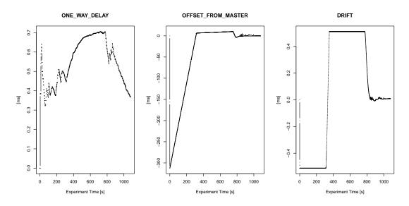
Figure 6.14.: Test Case 3; regular PTPd control system values for Subsystem 2. Initial Offset is comparably large.
