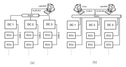
Figure 6.2.: Distributed system topology setup (Ruf et al., 2013a). Virtual LAN 0 is used for the experimentation in this thesis. Virtual LANs 810 and 820 feature live subsystem statistics in conjunction with LabVIEW.
