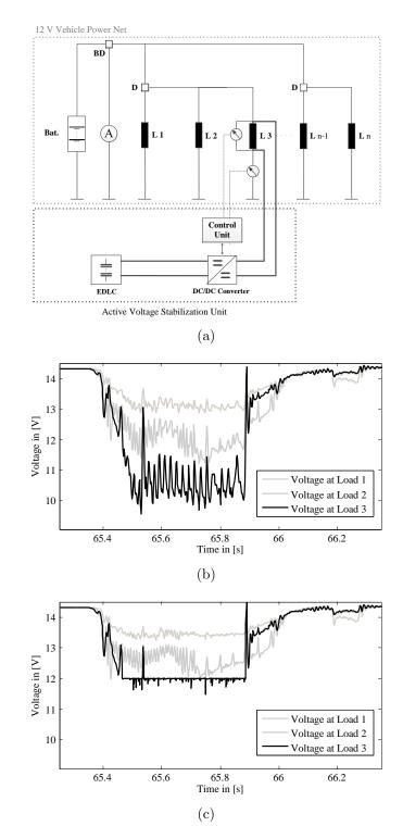
Figure 1.7.: Automotive power net and voltage stabilization example. Figures taken from Ruf et al. (2013b)
