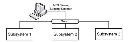
Figure 6.5.: Experiment Setup, Subsystems Connected via Ethernet
