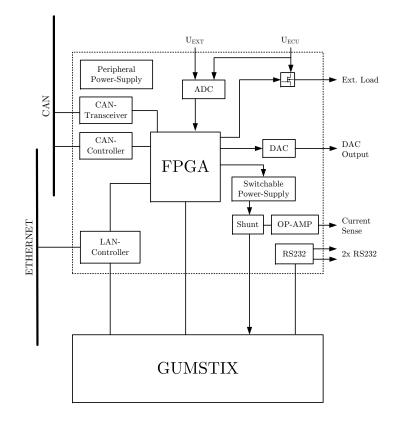
Figure 6.3.: Schematic of the Custom Platform Including the GUMSTIX Computer-On-Module (COM). The Figure is taken from Barthels et al. (2012c).
