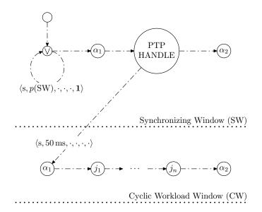
Figure 5.8.: PlannedPTPd—Plan for Master Node with Synchronizing and Cyclic Windows
