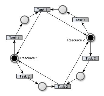
Figure 2.2.: Resource Processing in Tasks, Prone to Deadlocking
