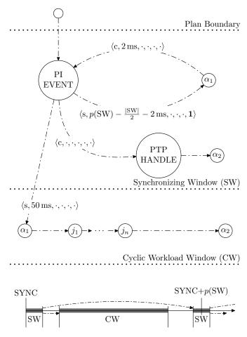
Figure 5.7.: PlannedPTPd—Plan for Slave Nodes with Synchronizing and Cyclic Windows
