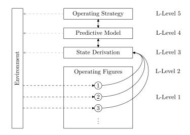
Figure 3.10.: Illustration of cybernetic control systems. Dashed lines are physical processes, solid lines are internal communication. Depicted are black arcs showing forward links, which are involved in deriving states, predictions, and strategies. Taken from Barthels et al. (2012a).
