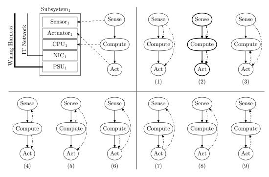
Figure 4.2.: Example of walking the solution space for scheduling within 1 subsystem  $E \in \mathcal{E}$ . ( $\rightarrow$  Integration Level); not depicted is the special case, where all software units are scheduled concurrently.
