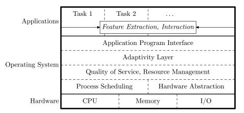
Figure 3.2.: System features are delivered by the application layer. Complex know-how and algorithms are involved and need abstractions.
