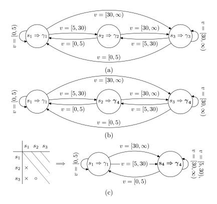
Figure 3.9.: Management complexity reduction through unifying plan generation. Illustration taken from Barthels et al. (2011)
