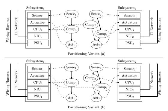
Figure 4.3.: Example Finding a Mapping and Afterwards Scheduling ( $\rightarrow$  Integration Level).
