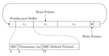
Figure 5.5.: Ring Buffer and Data Format Used in Logging Module
