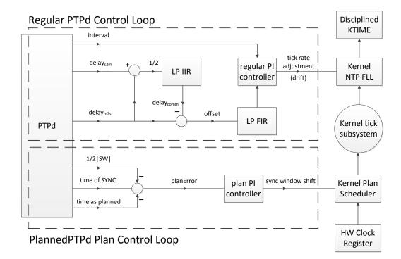
Figure 5.6.: Regular PTPd control loop as illustrated in Correll et al. (2005) together with extensions for PlannedPTPd version. To the right is the layered architecture of the scheduling, tick, and timing subsystem of the Linux kernel.
