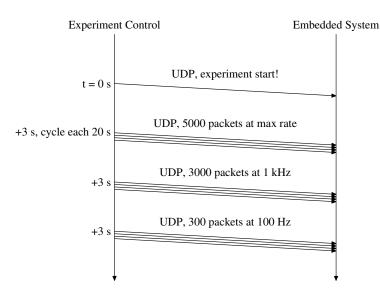
Figure 6.7.: Generated Network Packet Flow During Load Testing
