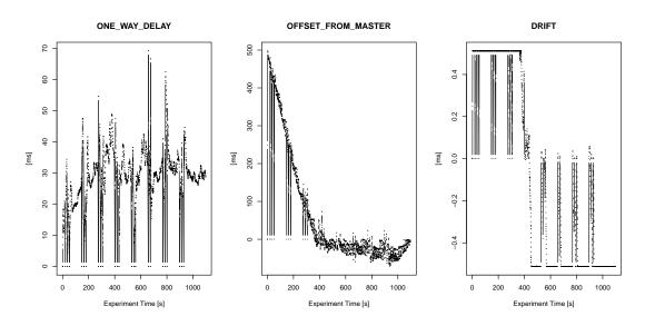
Figure 6.11.: Test Case 2; regular PTPd control system values for Subsystem 1 under presence of real time tasks. Measured values are discarded if they are off by more than 500 ms. Thus some values are intermittently clamped to zero. Due to the added noise, the time for convergence is significant.
