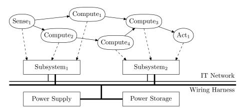
Figure 1.4.: Illustration of jobs interconnected by communication patterns and distributed onto embedded subsystems. Illustration taken from Barthels et al. (2011).
