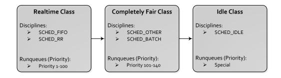
Figure 2.6.: Scheduling Classes as Being Implemented in Linux 3.0
