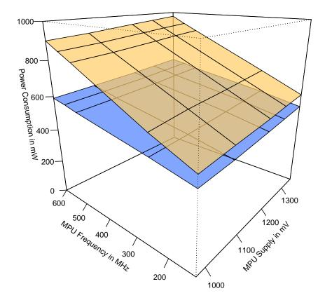
Figure 6.4.: Typical OMAP3503 MPU Power Consumption as Measured in Barthels et al.  $(2012 {\rm c})$
