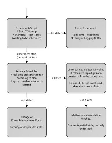
Figure 6.6.: Script as Used in the Plan Timing Experiment
