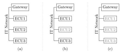
Figure 1.5.: AUTOSAR Mechanisms for Energy Efficiency in Electronic Control Units
