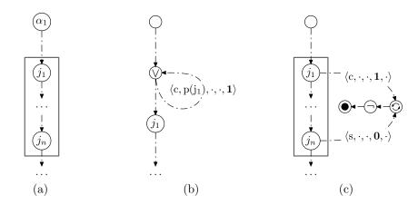
Figure 3.6.: Useful plan patterns for modeling common scheduling tasks. Figure a shows the ability to chain together job instances and choose the necessary power state for the series of jobs  $j_1, \ldots, j_n$  beforehand. Figure b models the notion of a cyclically scheduled job  $j_1$ . Figure c builds a critical section  $j_1, \ldots, j_n$ , within which switching in between power management plans is prevented.
