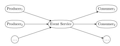
Figure 1.3.: Complex Interaction Pattern for Decoupling of Endpoints
