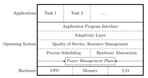
Figure 3.4.: Low Level Scheduling of Software Threads and Power ( $\rightarrow$  Hardware Abstraction) by Means of Power Management Plans
