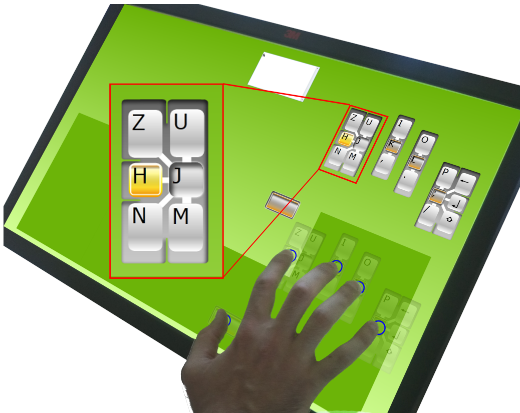
Figure 13.11.: The current position of each finger relative to the Gestyboard is visualized by a slider (see Letter 'H').
