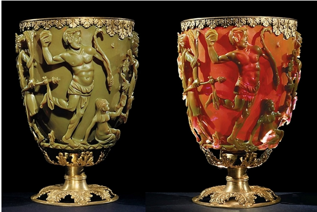
Figure 7.1 Lycurgus cup which appears green in reflected light and red in transmitted light [105].
