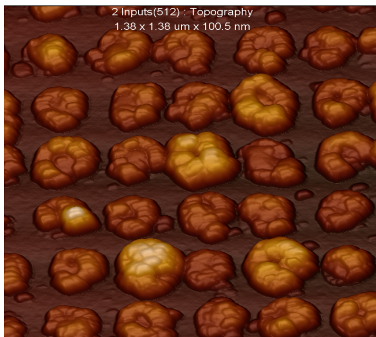
Figure 3.15 3D image of the nanopyllars showing detailed topography.
