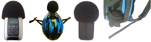
Fig. 1. From left to right: four-channel high quality audio recorder with wind shield and helmet mounting in 90^\circ angle of inclination, smart phone with windshield and positioning in the backpack. The additional GPS tracker was positioned inside the backpack ensuring sufficient satellite visibility.
