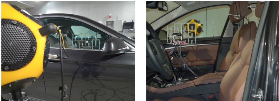
Figure 3 – The measurement setup with loudspeaker and sound pressure and particle velocity sensor array.
