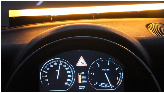
Fig. 4. ISPA User Interface: LED bar indicating obstacle distance together with suggested deceleration strength and instrument cluster with standard traffic symbol and distance indicator
