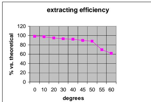
There are several methods to increase screw capacity with length and to reduce the necessary starting torque.
