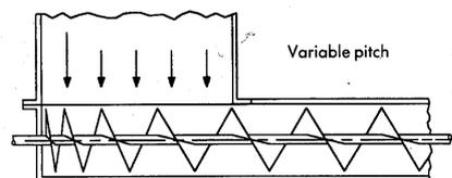
The minimum pitch must be no less than one-half the screw diameter (logging), the maximum pitch approx. one screw diameter.
