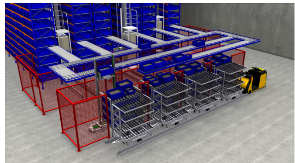
Fig. 2: Loading station for the automatic loading of tugging trains
