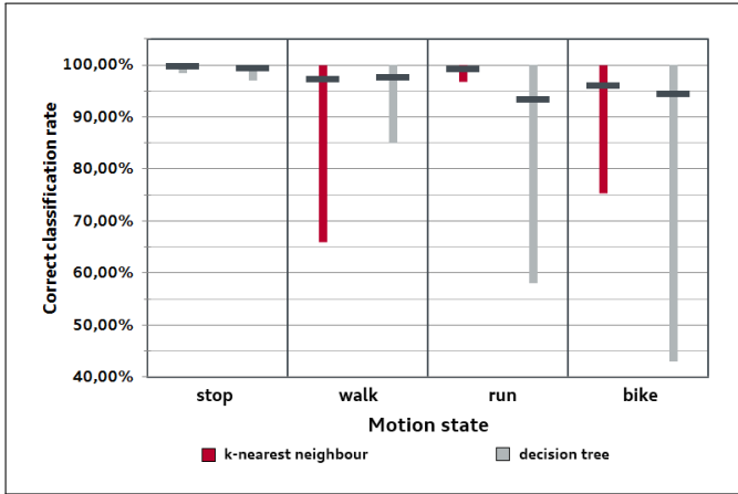
Fig. 2. Correct classification rate for different activities using a k-nearest neighbour algorithm and a decision tree.
