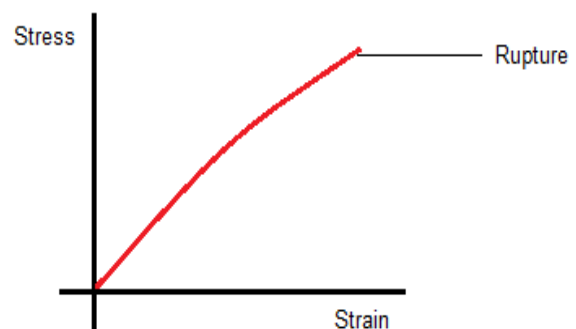
Fig. 8 Stress-strain-diagram of a brittle material such as stone or glass without change of rate of elongation prior to rupture (tensile stress applied).
