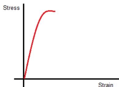
Fig. 10 Following Hook's Law, stress and strain are directly proportional during the initial phase in a stress-strain-diagram.
