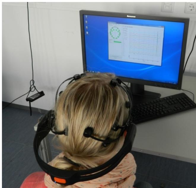
**Figure 6.12:** Fitting of the helm to achieve acceptable signal quality was a trial-and-error process which failed in the case of three participants
