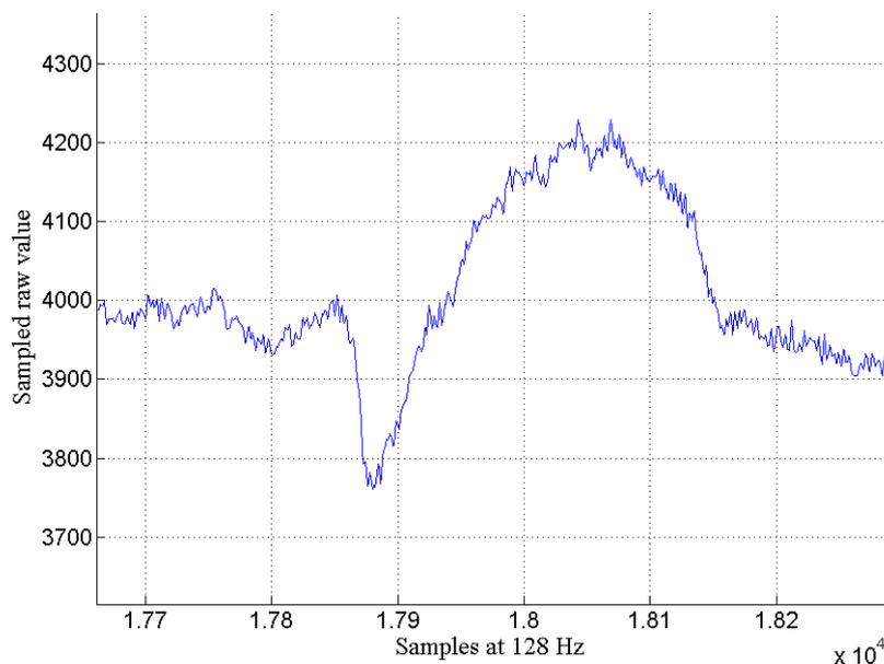
**Figure 6.14:** Long-term signal artifact which lasts several seconds before stabilizing
