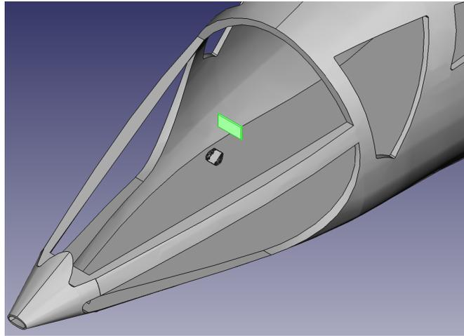
**Figure 4.12:** Possible placement of the heads-up display in the Innotruck's Cockpit
