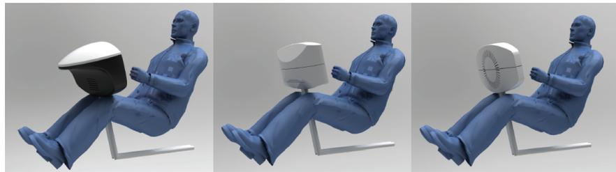
**Figure 4.4:** Proposed designs of the central console element
