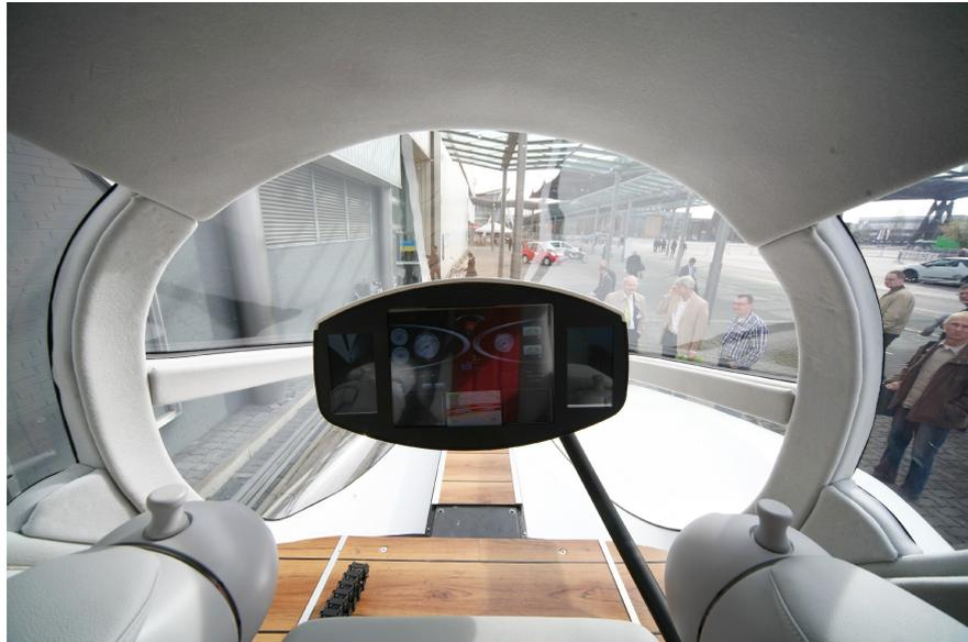
**Figure 4.2:** A look at the main human-machine interfaces in the Innotruck: The virtual dashboard in the front and the side sticks left and right
