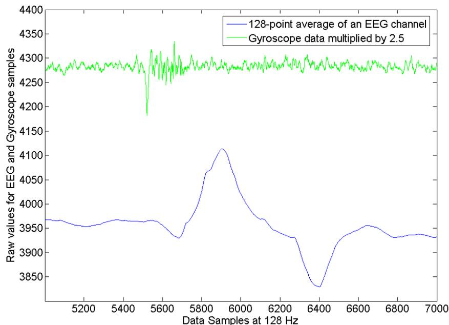
**Figure 6.13:** Scaled gyrosopic data and raw EEG data showing how increased gyrosopic Y activity(green) resulted in moving EEG average(blue)
