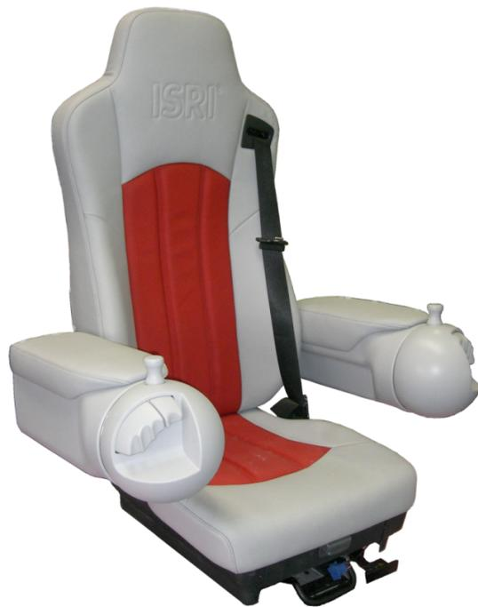
**Figure 4.13:** The driver's seat with two integrated spherical side sticks
