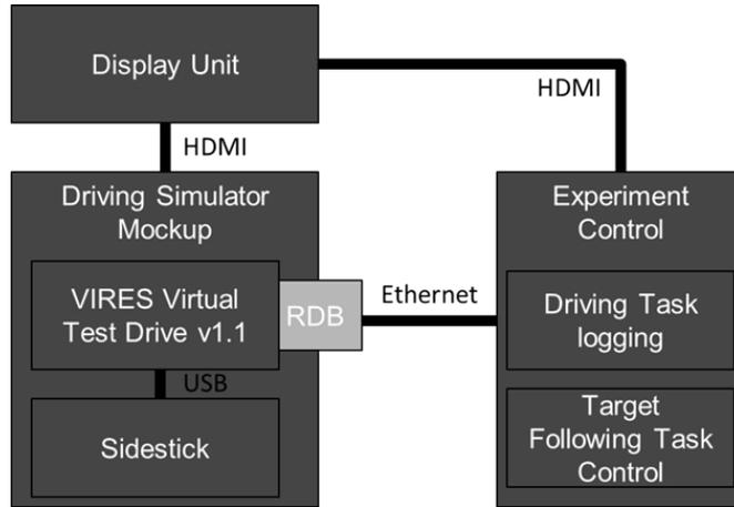
**Figure 6.6:** Data flow between software and hardware components in the driving simulator
