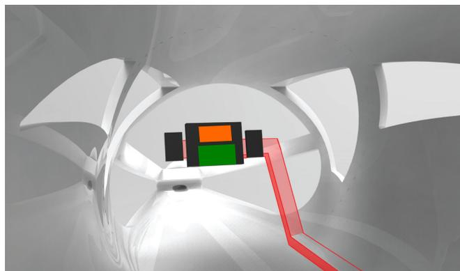
**Figure 4.11:** Study on replacing the central console with a tablet(green surface) and a heads-up display(orange surface)
