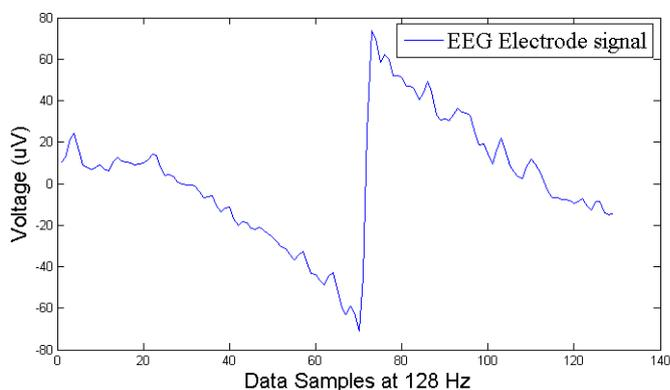
**Figure 6.15:** Short-term effect of electrode slippage which stabilized in timeframe of one second
