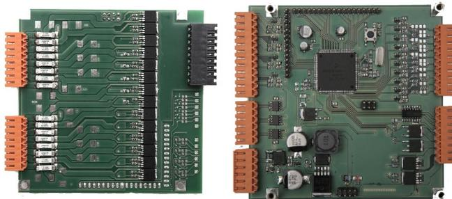
**Figure 4.7:** The vehicle control unit which serves as a gateway between the central console and the Innotruck
