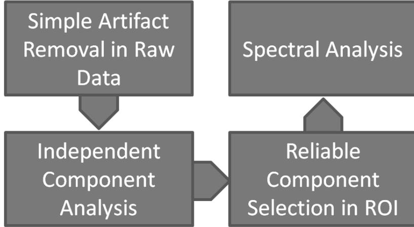
**Figure 6.17:** Basic blocks of the signal processing pipeline of the algorithm’s on-line phase
