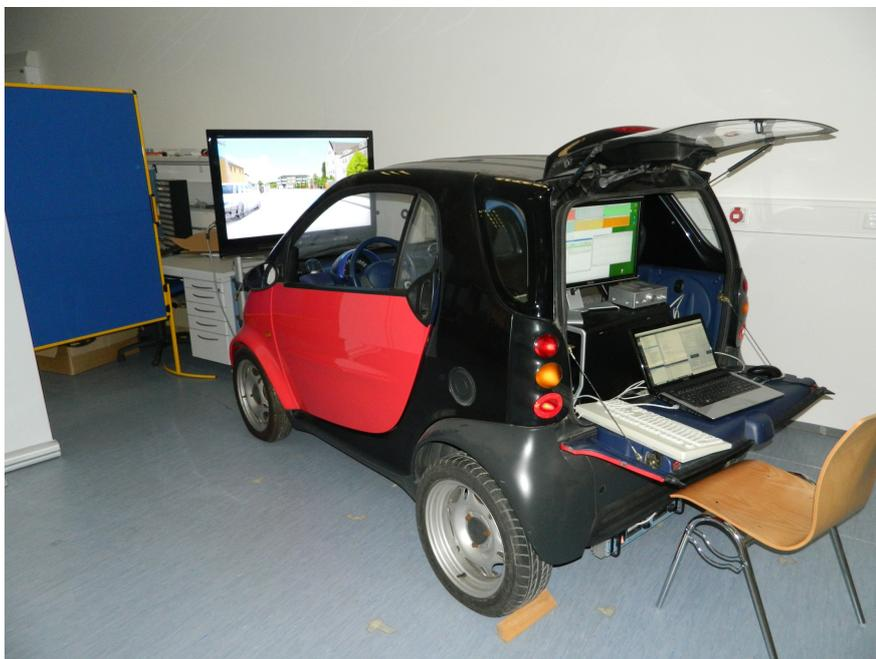
**Figure 6.1:** VIRES Virtual Test Drive driving simulator with vehicle mockup
