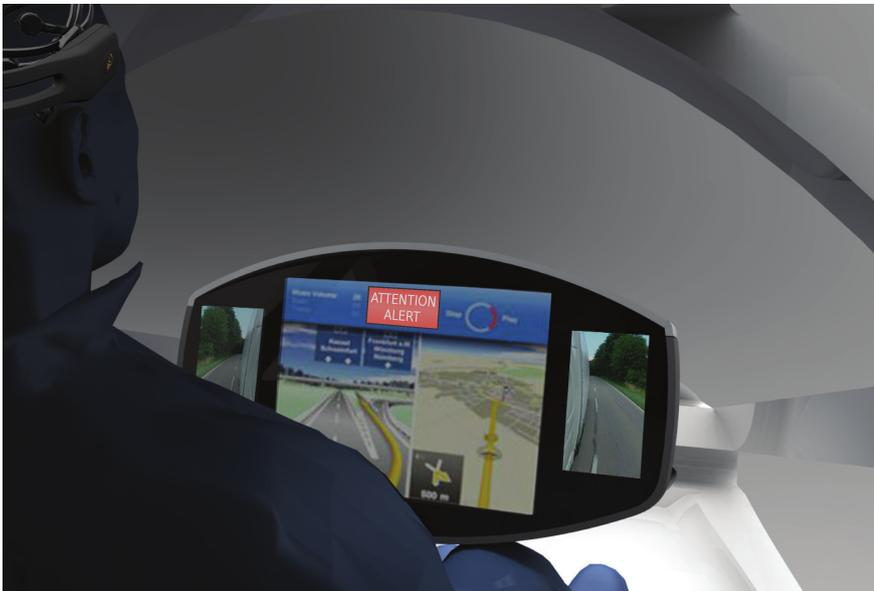
**Figure 6.19:** The EEG helm can be comfortably worn while the prototype vehicle is driven with conventional human-machine interfaces(Image by Juan Jose Gonzalez Herrero)
