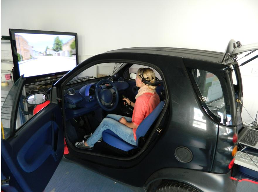
**Figure 6.2:** A participant with fitted Emotive EPOC wireless EEG helm inside the driving simulator
