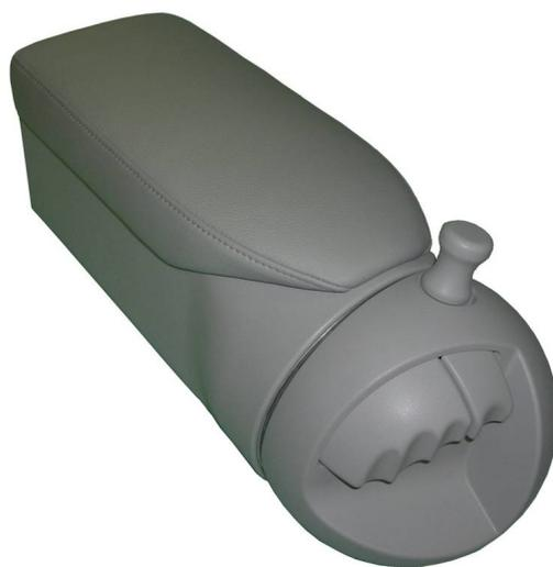
**Figure 4.14:** One of the two spherical side sticks integrated in the driver's seat
