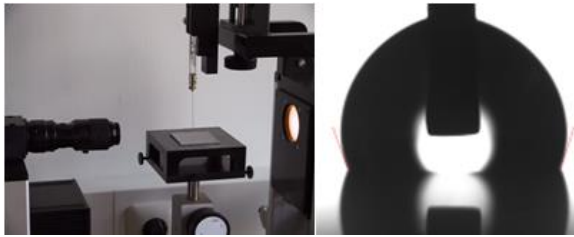
Figure 4: Contact angle goniometer (left) and drop on hydrophobic surface (right)
