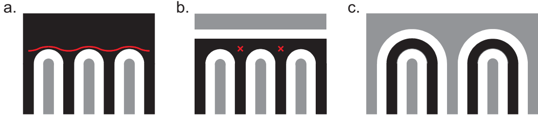
Figure 3.15: Variations for contacting the microstructure electrodes underneath the perimeter electrode. a. This simplest variation works fine on the side of the microstructure where the black electrode has the opposite polarity as the perimeter electrode. However, when the black electrode has the same polarity as the perimeter electrode, a zero-field region indicated by the red line exists on the surface of the electrode, resulting in holes in the electric trap. b. The region of zero electric field on the microstructure surface can be eliminated by adding an additional electrode with the opposite polarity as the perimeter electrode above the electrode with the same polarity as the perimeter electrode. However, the electric field strength is still substantially weakened in the vicinity of the red crosses, and the holes in the trap thus effectively remain. c. The holes in the trap can be almost completely eliminated by bending the microstructure electrodes with the same polarity as the perimeter electrode around and contacting them in a single location at the side of the trap.
