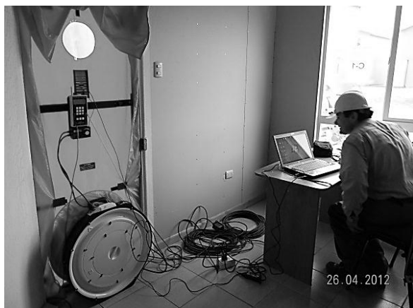
Figure 1: CITEC UBB staff performing a Blower Door Test
