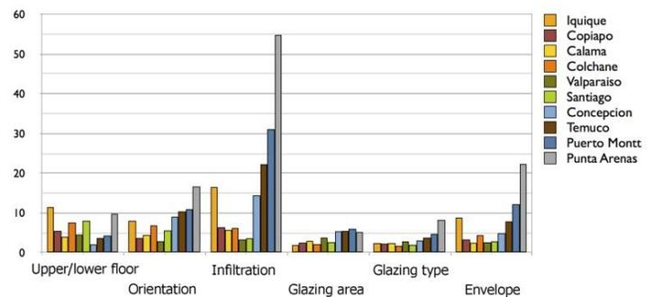
Figure 4: influence of design parameters - difference in energy demand (kWh/m<sup>2</sup> y)
