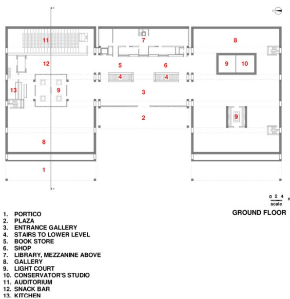
Figure 4: Ground floor plan of the Kimbell Art Museum (original source for plan: [11], redrawn by the author).
