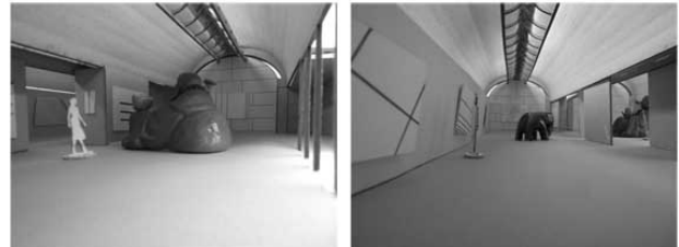
Figure 8: The visual environment in the Kimbell Art Museum as in the pictures of physical model testing under artificial sky (physical model and pictures by the author).
