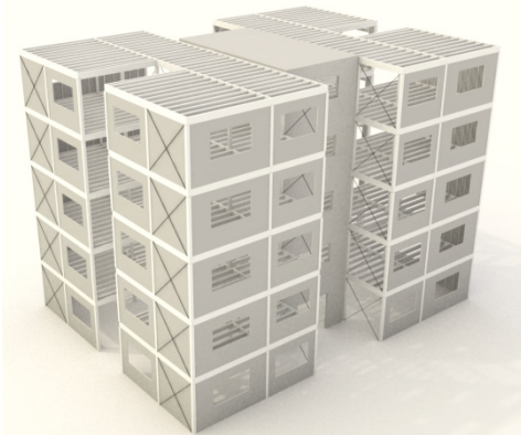
Figure 4: whole building structure with System 3
