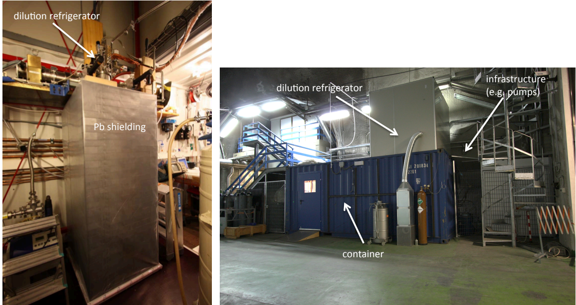
Figure 3.1: The test cryostat installed in the underground laboratory of the LNGS in Italy. The facility is dedicated and optimized for the operation of one CRESST-detector module under realistic operational conditions. Left: The dilution refrigerator inside the Pb shielding. Right: Outside view of the container which houses the test cryostat.
