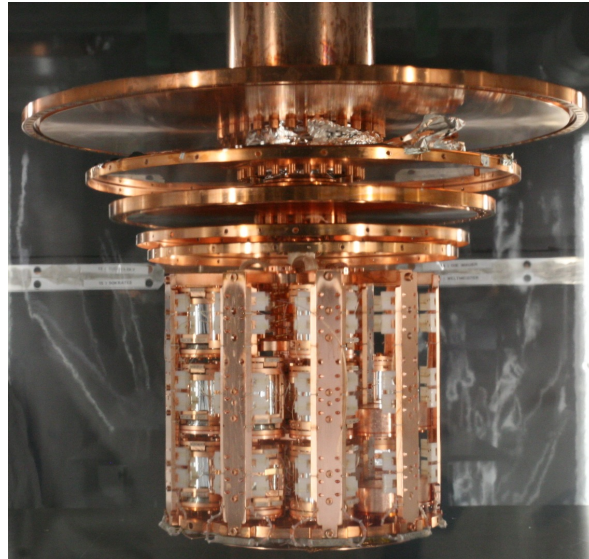
Figure 2.17: Detector volume (“carousel”) of the CRESST experiment. The picture shows the fully mounted setup for CRESST run33. In total, 18 detector modules are mounted. Two of those are prototype detectors with a fully-scintillating detector design developed in this thesis (see chapter 3.5).
