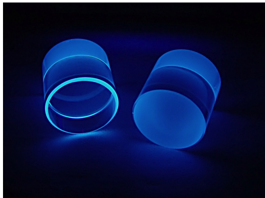
Figure 2.1: Picture of standard CRESST-size \text{CaWO}_4 crystals under UV-light irradiation. The front surface of the left crystal is polished (bevelled edges) while the right one is roughened which visibly homogenizes and enhances the light output through this surface.
