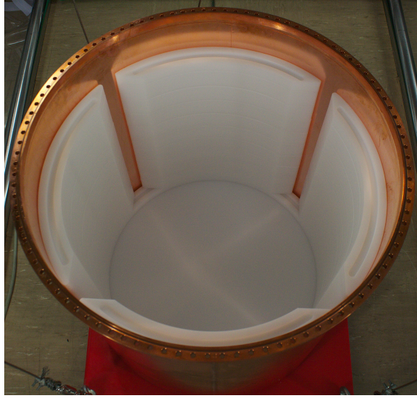
Figure 2.18: Inner PE shielding of \sim 3 cm thickness mounted in the inner vacuum vessel of the CRESST cryostat. The gaps in the PE allow to perform neutron calibrations with sources from outside the cryogenic part. The gaps are closed by an additional layer of PE at the outer part of the cryostat, however, still inside the Cu shielding. The outer PE parts can be removed for calibration during the experimental run.
