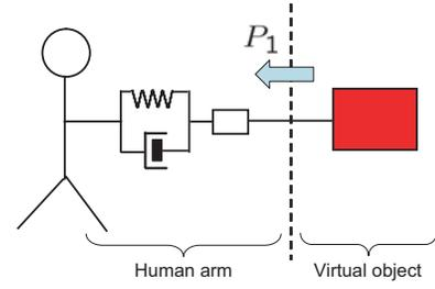
Figure 4: Mechanical model of single human operator interacting with the virtual object
