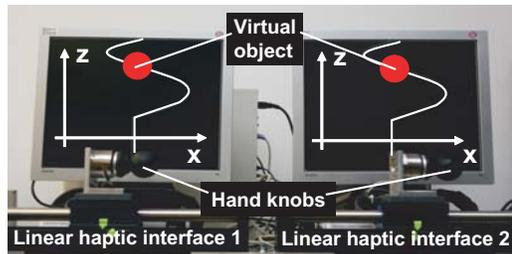
Figure 2: Experimental setup consisting of two linear haptic interfaces (linked by the virtual mass) and two screens with the graphical representation of the tracking path
