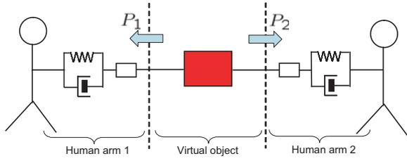
Figure 5: Mechanical model of interacting couple
