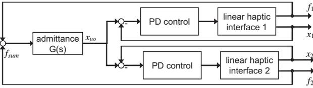
Figure 3: Position-based admittance control of the linear haptic interfaces in the dyadic condition
