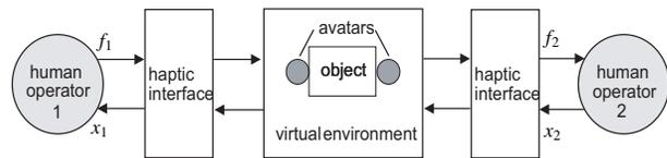
Figure 1: Interaction with virtual environment via haptic interfaces in case of the dyadic condition
