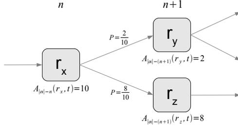
Fig. 3. Sampling for a fair routing in step  $n$ . The number of feasible paths  $A$  that are still left to reach the target determine the probability of a hop to be taken in  $n + 1$ .
