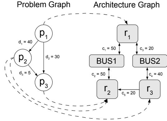
Fig. 1. Specification Graph: Edges in the problem graph are annotated with demands  $d_e$ . Edges in the architecture graph are annotated with capacities  $c_e$ .
