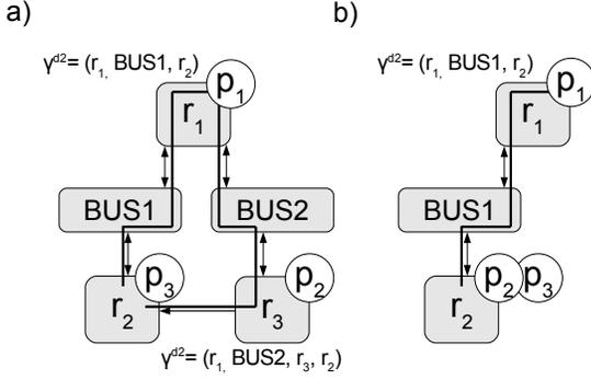
Fig. 2. Implementations of the specification in Fig. 1: Implementation a) offers two paths to establish the data dependency  $d_2$  while implementation b) only offers one possible path, because resource  $r_3$  and  $BUS2$  are not allocated.
