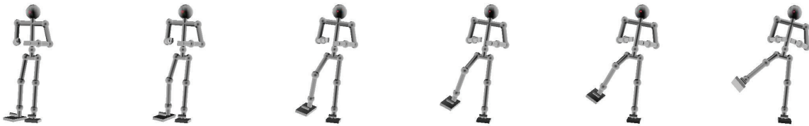
Fig. 12. Frames from the generated sequence of the right kick raise (RKR) abstracted motion primitive.
