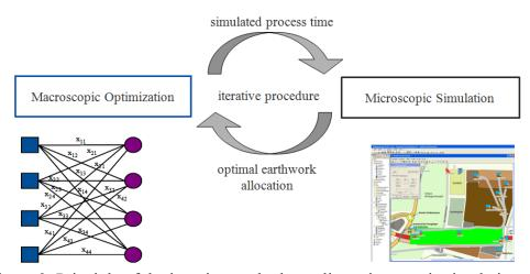
Figure 2: Principle of the iterative method coupling microscopic simulation and macroscopic optimization
