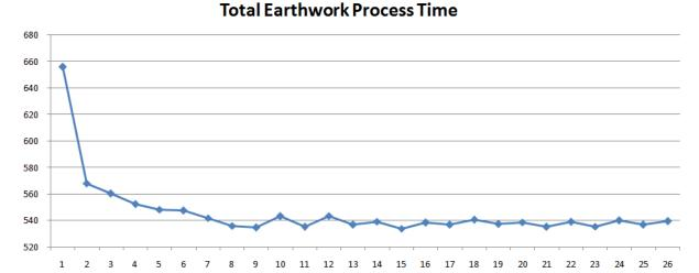
Figure 5: Changes of total earthwork process time [h] (vertical direction) during 26 iteration steps (horizontal direction)
