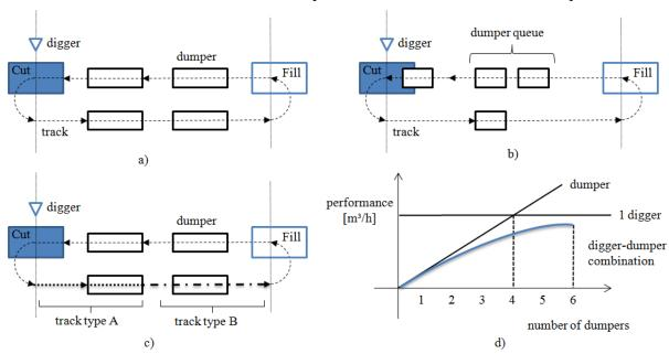
Figure 1: Detailed modeling of earthwork processes under consideration of microscopic conditions; a) ideal process b) waiting queue c) properties of tracks d) non-linear working performance in earthwork processes
