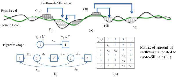
Figure 3: Schematic representation of modeling the earthwork allocation problem with a bipartite graph; the optimal cut-to-fill allocations can be represented using a transport matrix
