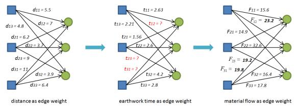
Figure 4: Converting the earthwork process time in material flow for each cut-to-fill pair
