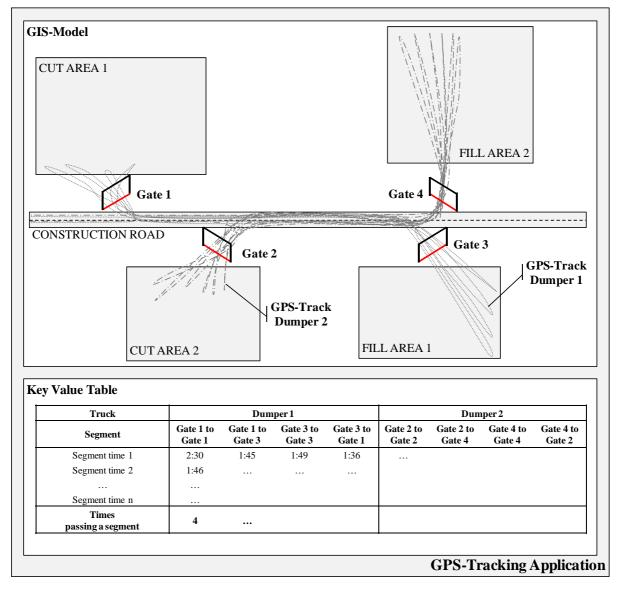
Figure 3: Gate-concept for processing GPS-tracks to key values for the construction progress
