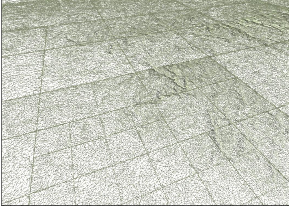
Figure D.2 — Scene composed of multiple W3DS GetTile requests, rendered in wireframe mode
