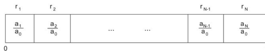
Figure 2.6: Illustration of the correlation between the drawn number x_1 \in ]0; 1] and resulting reaction r_j .
