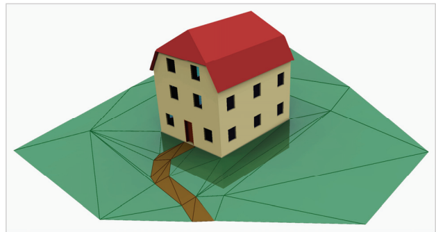
Figure 9. Consistent integration of the datasets shown in figure 8 is facilitated by detailed semantic information coherently structured with geometry and topology.
