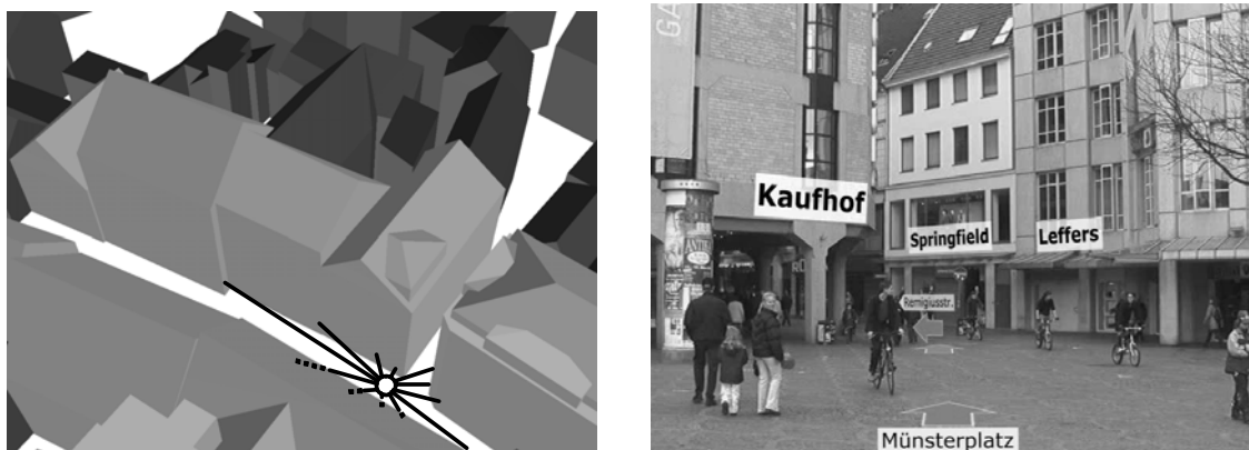
Figure 11. 3D city models provide orientation and guidance: determination of the current position using range finders and a 3D city model (left), and background and wayfinding information presented by virtual 3D banners and signposts help to guide rescue teams (right; example taken from pedestrian navigation).
