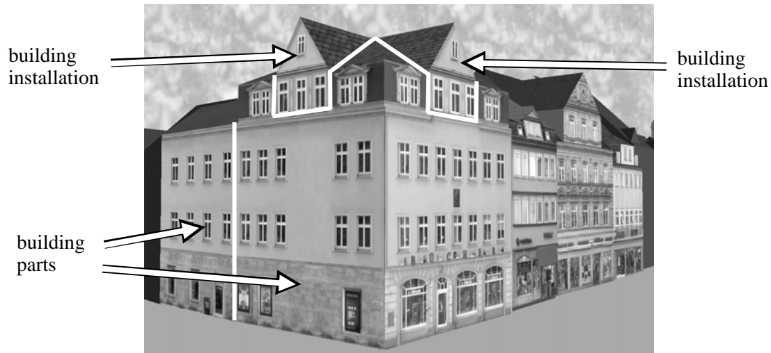
Figure 6: Illustration of a LoD2 building. It consists of two building parts with different heights. The right part has two dormers represented as building installations.
