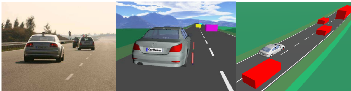
Figure 2/3: Real and simulated test scenario „Changing lane into a convoy“
