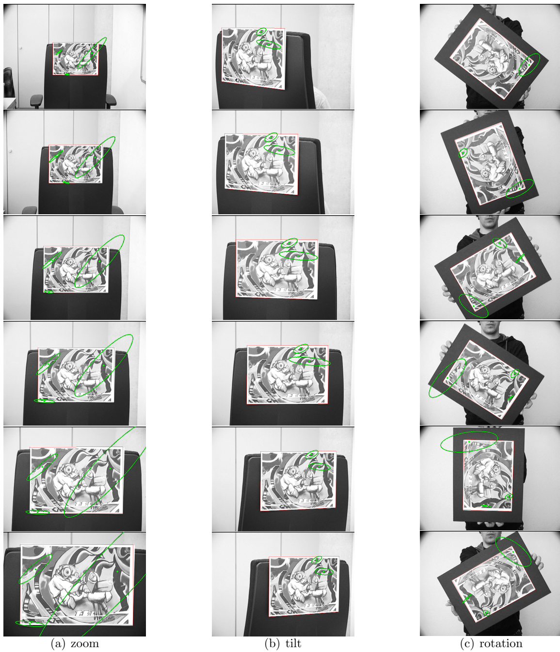
Figure 3.33: Three image sequences with different perspective distortions, and the evolution of the covariance for selected SIFT features. A small green dot marks the feature locations, the ellipses indicate their estimated covariance. (Image reproduced from [Zei09])
