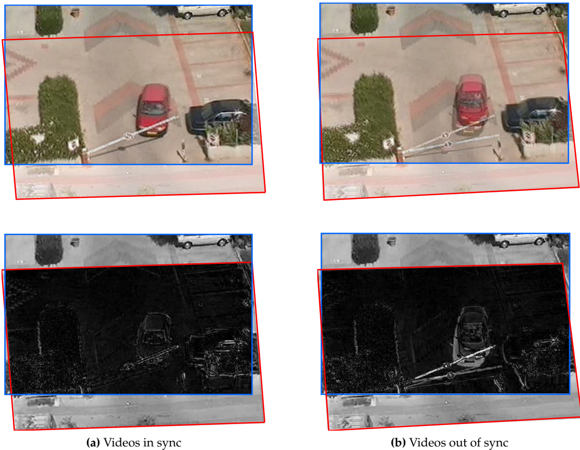
Figure 2.2: Example for intensity-based video synchronization: Two telephoto views of the same scene are warped and superimposed in the top row. Their gray level difference is shown below. (a) For simultaneously acquired frames, the alignment is rather accurate. (b) Between frames from different time instants, however, dynamic objects cause significant intensity differences. (Source images from [CI])
