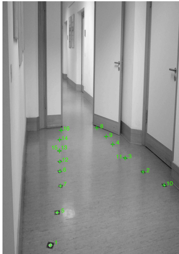
Figure 3.23: Image captured with a Panasonic DMC-FX1 at original resolution 1536 \times 2048 pixels. The detected SURF markers are labelled according to the ranking in Figure 3.24.
