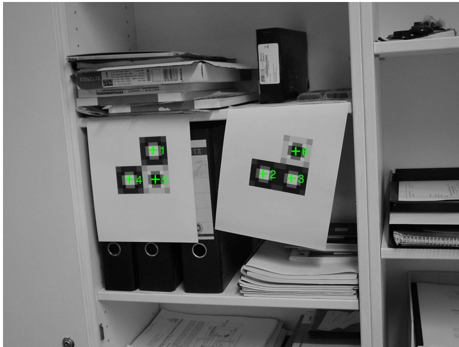
Figure 3.26: Two out of eight possible 3-bit marker arrays photographed with a Sony DSC-S85 at resolution 2272 \times 1704 pixels. The location of the six SURF features which yielded highest detector response are displayed as green crosses.
