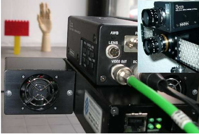
Fig. 2. Piggyback assembly of PMD and color CCD.
