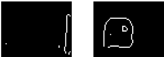
Fig. 8. Canny edge detector used for segmentation: vanishing (left) and nearing obstacle (right)
